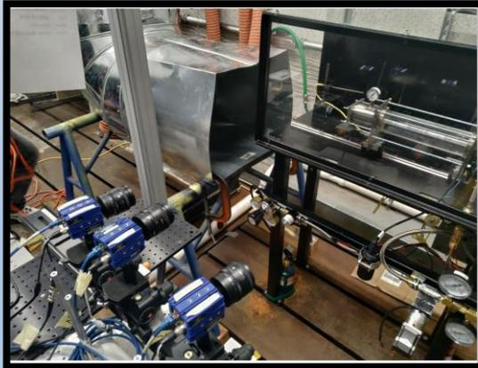
Imaging was also conducted to observe the **exhaust and combustion chamber** during test runs of the rocket.
