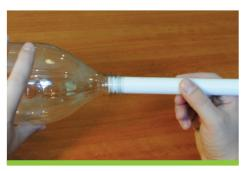
**Step 9:** Secure the pipe to the bottle using a 4" long piece of duct tape.
