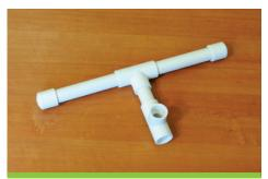
**Step 5:** Insert one end of a 12" pipe piece into the other end of the PVC tee connector.
