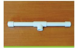
**Step 3:** Insert the 2" pipe piece into the open connection of PVC tee connector.
