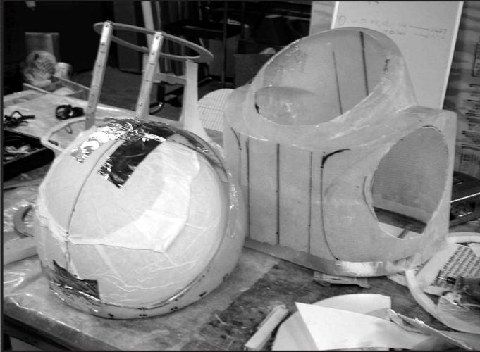
Shown here are the forms for the helmet and hard upper torso for the North Dakota Experimental Planetary Space Suit.
