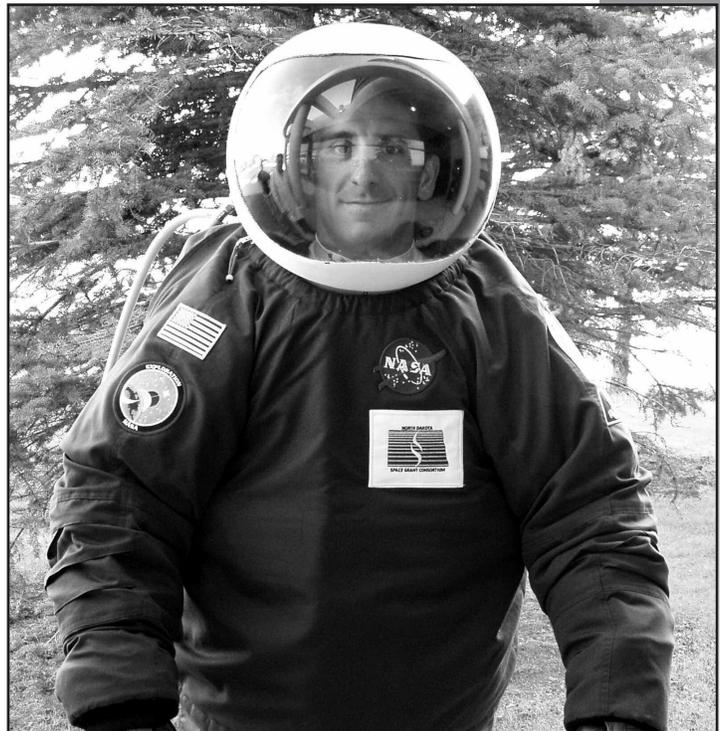
Fabio Sau, graduate student in Space Studies at UND, tests the environmental system of space suit while wearing the inner garment, the outer garment and the helmet.
