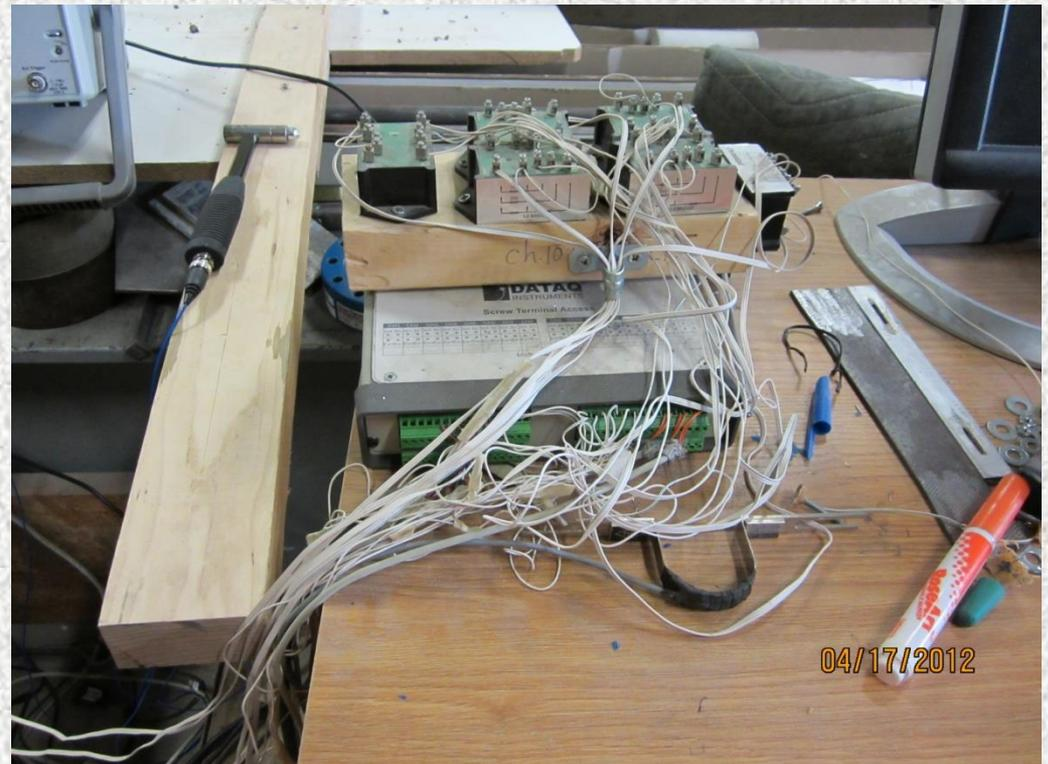
Dataq Instruments for strain gage data collection.
