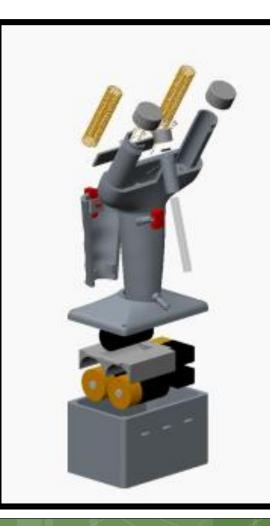
Left: Exploded view of final wand rendering. Note: View is from rear left of device.
