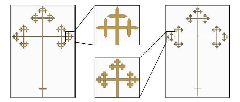
The fourth order fractal with pointed ends. The 4<sup>th</sup> order fractal has 81 nodes. The fifth order fractal with square ends. The 5<sup>th</sup> order fractal has 243 nodes.
