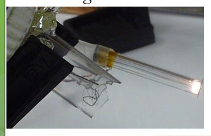
Electron gun with tube of nitrogen connected. Two copper wires in tubing connected by the tungsten filament and to the power supply. To prevent separation of the wires that would cause the filament to break, the wires are secured by an additional glass piece at the front (right) end of the tube.
