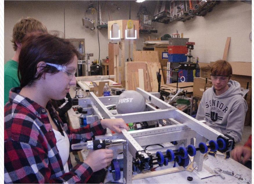
Using a pneumatic riveter.
